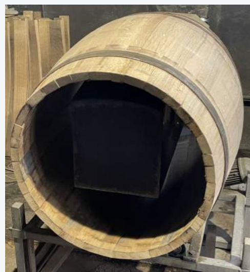
Convection toasting being used for the "Radiant White and Red" toasts.
