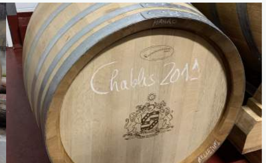
45 mm thick stave 500L puncheon in Chablis.
