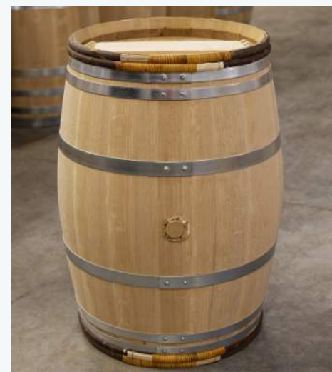
Finished 225L Bordeaux Château barrel.
