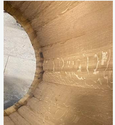
Noisette color of the inside of a DAMY barrel after the 2 hour super light long "Imperial" toast.
