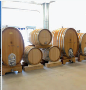
Schneckenleitner casks including 500L 45 mm puncheons.
