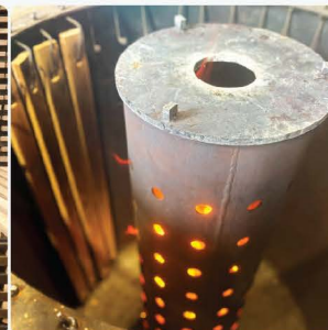
Fire-toasted staves done by hand over a live flame, just like toasting barrels.
