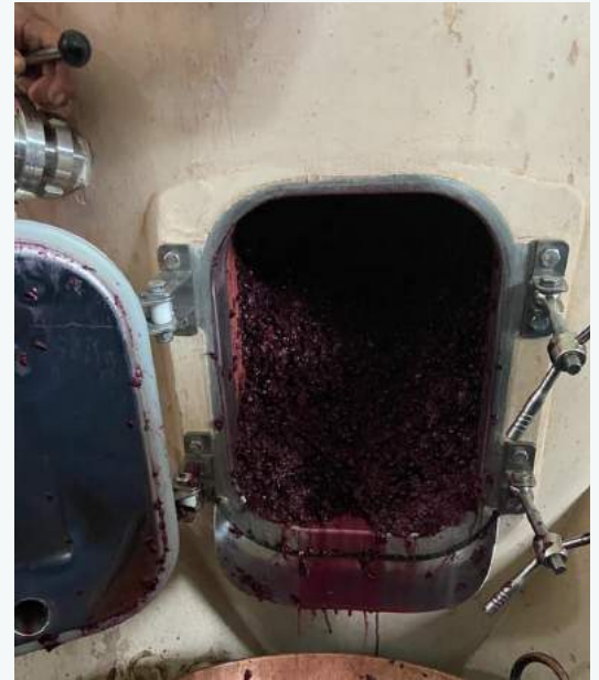
Extremely useful external opening door for removing ferments.
