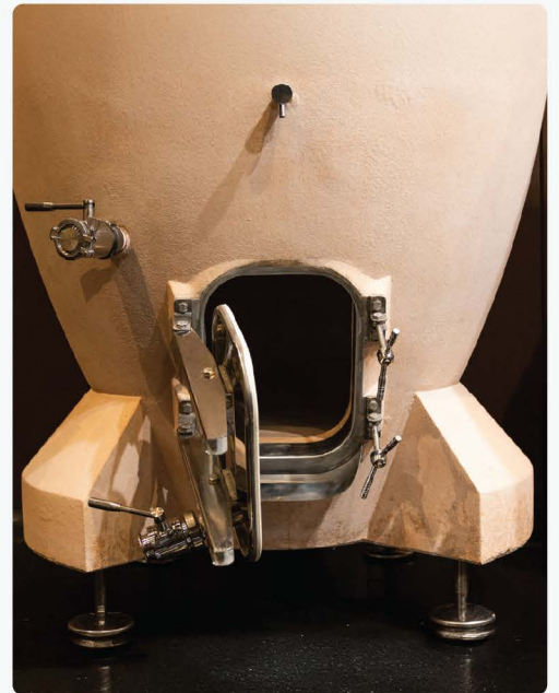
Featuring winemaking accessories such as a door for removing red ferments.
