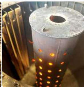
Fire-toasted staves done by hand over a live flame, just like toasting barrels.
