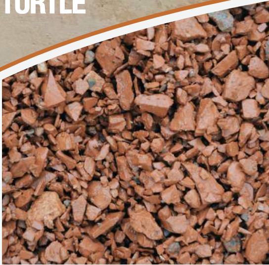
Terracotta and other Italian stone aggregates that make Cocciopesto.
