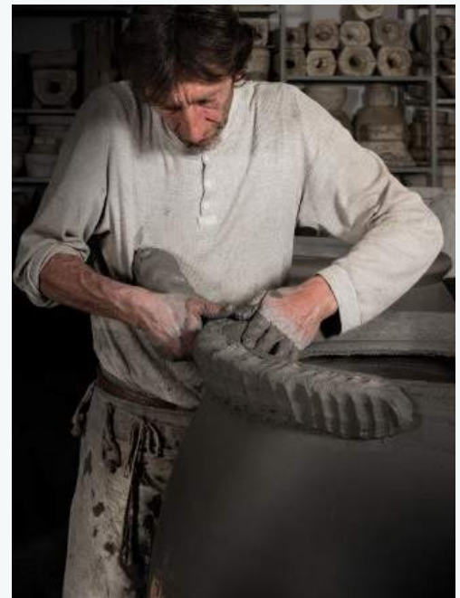
Colombino technique being applied to make a classic amphora.
