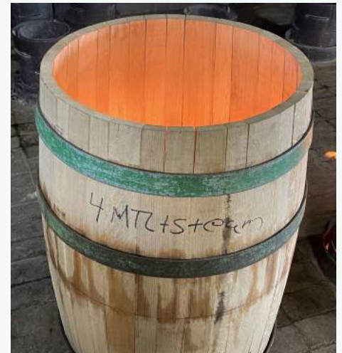
Master Coopers USA steam bent barrel.
