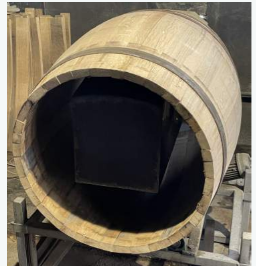
Convection toasting being used for the "Radiant White and Red" toasts.
