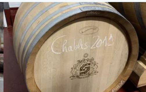
45 mm thick stave 500L puncheon in Chablis.
