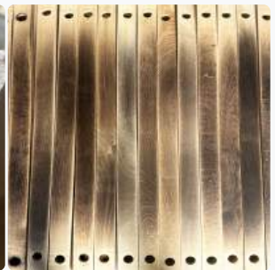
An assortment of different fire-toasted staves.
