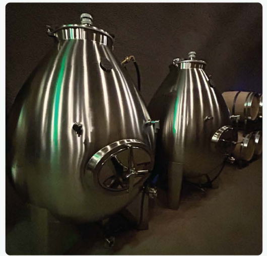
2x 1,500L Egginox for whites at Knight's Bridge in the Alexander Valley.
