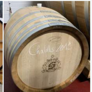
45 mm thick stave 500L puncheon in Chablis.
