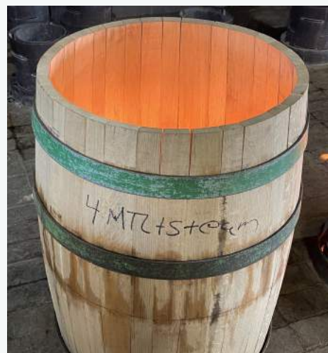
Master Coopers USA steam bent barrel.
