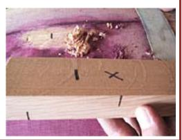
**3.** Then use a sharp-bladed chisel to make a hole BEFORE the grain exits. The wood chisel needs to cut ACROSS the grain where the wine is seeping, never lengthwise (this would aggravate the problem).
