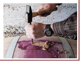
**4.** Cut the wedge width to the proper size and insert it into the hole you have made. Gently tap it into position; the wedge should fit snuggly.
